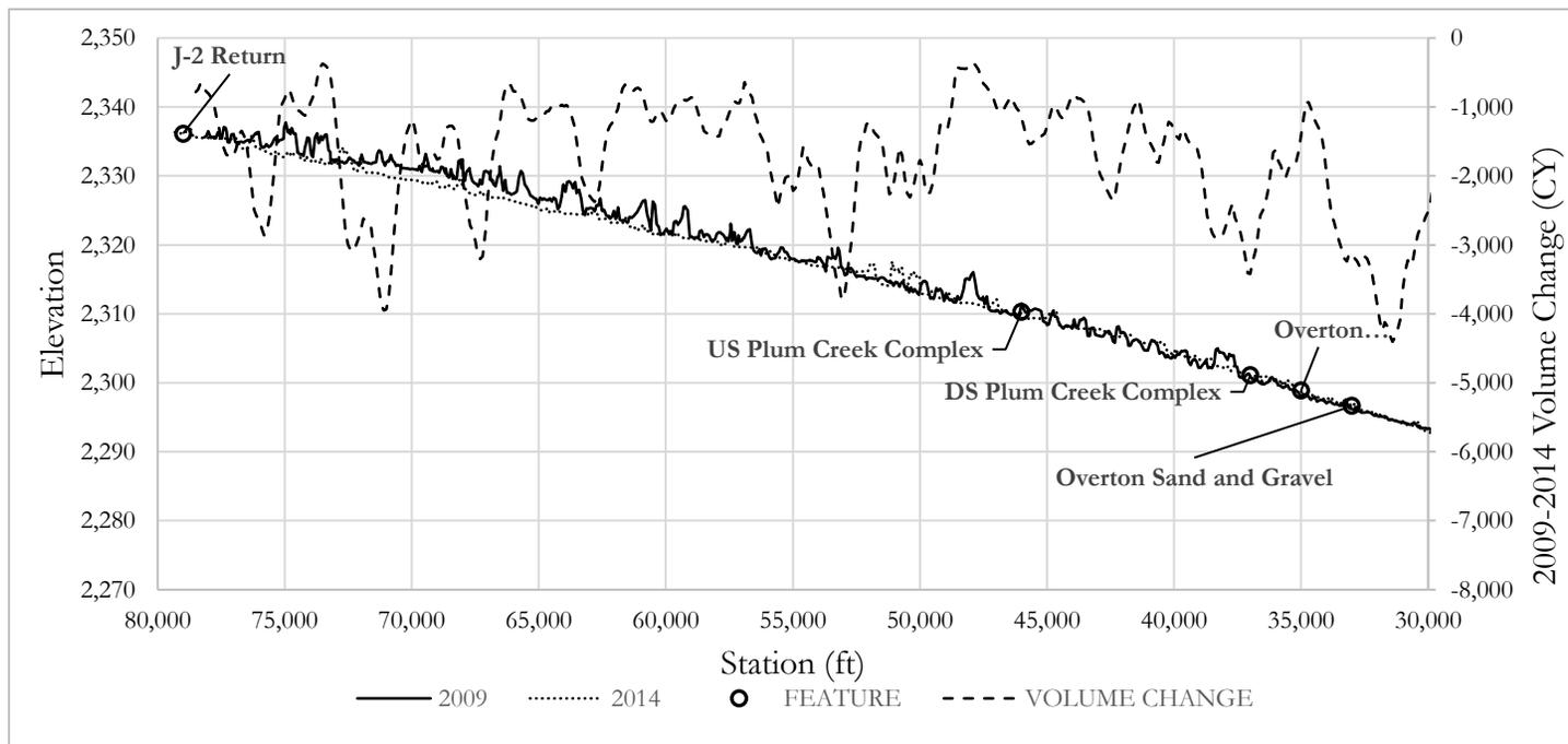
**Figure 3.** 2009 to 2014 longitudinal profile and volume change for the reach from J2 Return to Overton bridge. Volume change in the reach immediately downstream of the J-2 Return is caused by channel incision. Further downstream, volume change is due primarily to channel widening.
