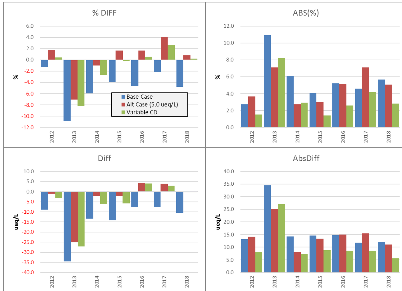
Figure 7.4. Charge balance by year across all lakes under three different assumptions for the organic charge density. “Base Case” applies a value of 7.5 \mu\text{eq}/\text{mg C} (as per the STAR, KAA and EEM). “Alt Case” applies a value of 5.0 \mu\text{eq}/\text{mg C} (as per the sensitivity analyses described in the text). “Variable CD” applies the lake-specific estimate of organic charge density that produces the best charge balance (as described in the text; values between 0.5-10.0 \mu\text{eq}/\text{mg C} ). The four metrics of charge balance are: %DIFF = average of the relative difference (%); ABS(%) = average of the absolute value of the relative differences (%); Diff = average of the absolute differences ( \mu\text{eq}/\text{L} ); AbsDiff = average of the absolute value of the absolute differences ( \mu\text{eq}/\text{L} ).
