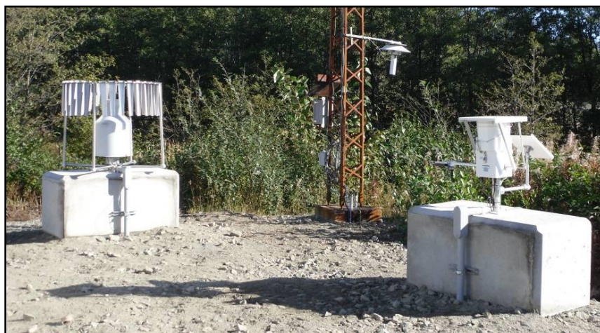
Figure 7. Haul Road wet deposition monitoring location (Station #6, NADP ID BC22), showing electronic recording rain gauge (shown at left) and a wet deposition collector (at right).
