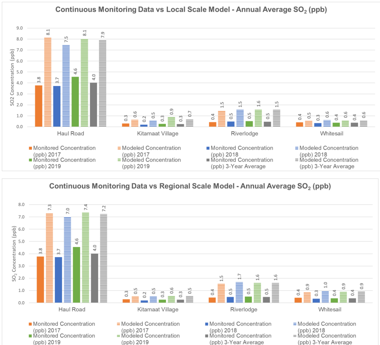
Figure 8. 2019 Monitored annual average data compared to modelled concentrations.
