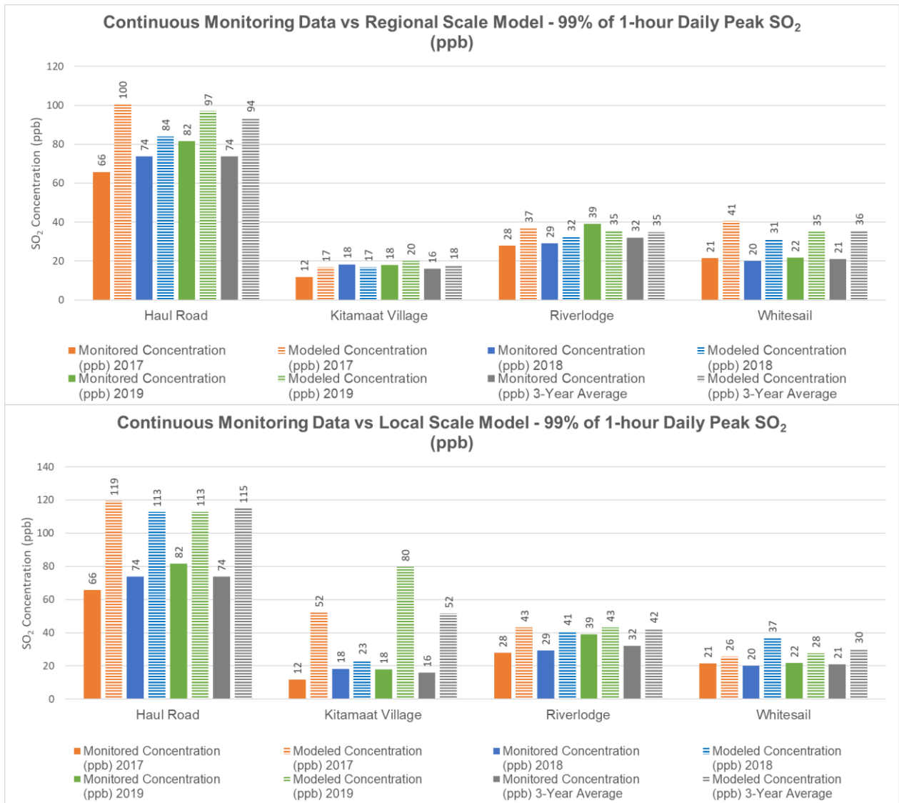
Figure 9. 2019 Monitored 1-hour data compared to modelled concentrations.
