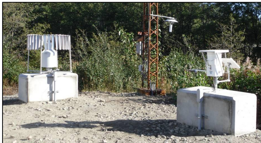
Figure 7.4-4: Haul Road wet deposition monitoring location (Station #6, NADP ID BC22), showing electronic recording rain gauge (shown at left) and a wet deposition collector (at right).
