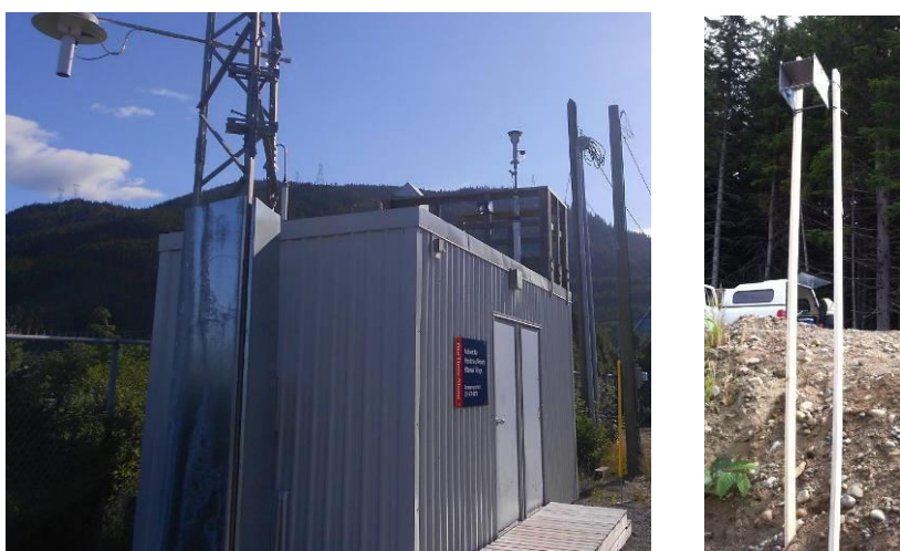
Figure 7.3-2: Example photos of continuous and passive monitoring for air quality at (left) Kitamaat Village continuous monitoring station, and (right) Low Spot passive monitor.
